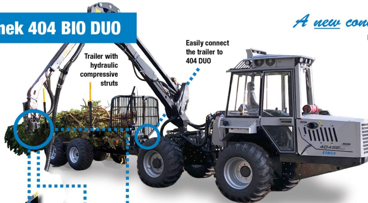
Trailer with hydraulic compressive struts
